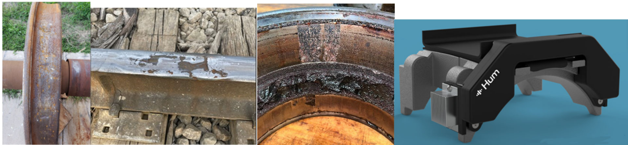
Figure 1: Onboard Sensing (Left to Right): Detected wheel defect, detected rail defect, detected bearing defect, bearing adapter with load sensing and energy harvesting based on UTCRS licensed technology.
